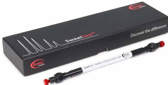
SweetSep™ columns for separation of all classes of carbohydrates by HPAEC(PAD)-MS
