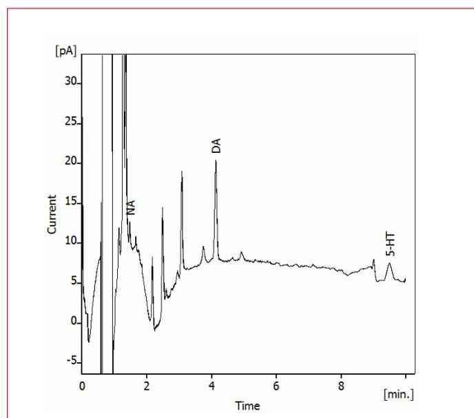
**Figure 11:** Chromatogram of rat brain Nucleus accumbens dialysate, acidified during collection with acetic acid (10 mmol/L final concentration). Injection volume 5  $\mu$ L. Conditions as in Table 3, but with the use of a  $\mu$ VT-03 flow cell.
