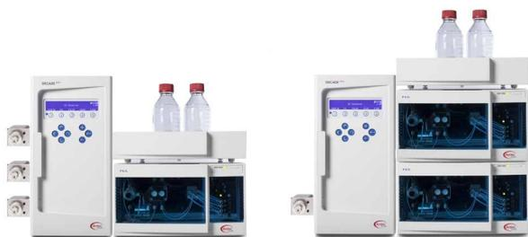
Additional versions of ALEXYS Analyzer for OMD. Left: High Throughput version, where three valves and one pump with a flow splitter are used for three HPLC channels running in parallel. Right: Parallel Channel version, where 2 pumps are needed for the two independent analyses running in parallel. The Time Resolution and single channel version are depicted in Fig. 2.
