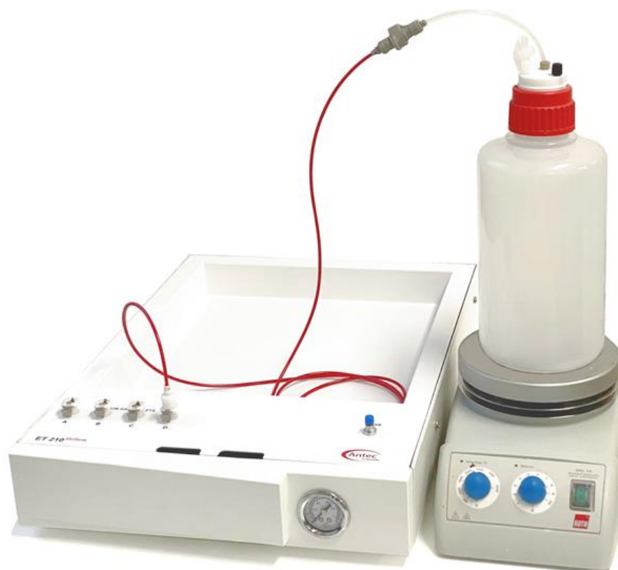
Fig. 9. Set-up for mobile phase preparation using inert gas sparging.
