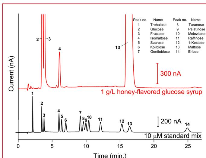
Figure 7. Overlay of chromatograms of: 10  $\mu$ L injection of 1g/L honey-flavoured glucose syrup sample (red) and a 10  $\mu$ L injection of 10  $\mu$ M standard mix (except nigerose) in DI water (black).
