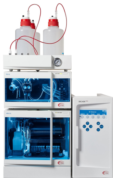
Figure 5. Recommended instrument configuration for this application: the ALEXYS Carbohydrate Analyzer The system consists of a P6.1L pump with integrated Solvent Switch Valve (SSV) capable of running step gradients, an AS6.1L autosampler, an ET 210 Eluent tray for nitrogen blanketing, and the DECADE Elite electrochemical detector. A CT 2.1 column oven with broad temperature range can be added optionally. The ALEXYS Carbohydrate Analyzer can be fully controlled by different Chromatography Data System (CDS) software: DataApex™ Clarity™ CDS (version 8.3 and up) or Thermo Scientific™ Chromeleon™ CDS (version 7.2 SR 5 and up).
