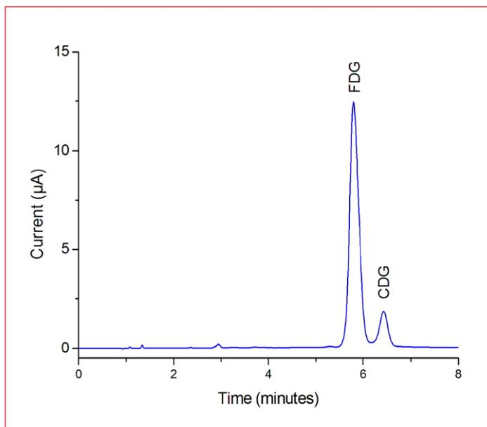
**Figure 6:** Chromatogram of 1.0 mg/mL FDG & 0.1 mg/mL CDG in mobile phase (1 µL injection of system suitability solution as described in the USP monograph).
