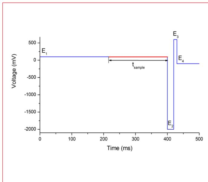
**Figure 3:** 4-step PAD potential waveform for the detection FDG and impurities.
