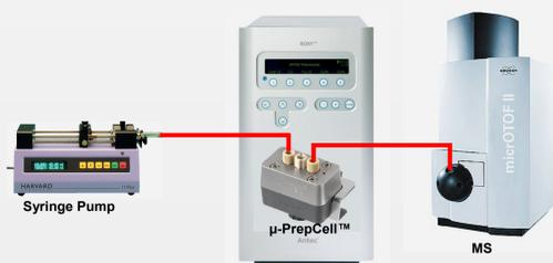
Figure 2. Instrument configuration of on-line ROXY™ EC system (Antec) coupled with mass spectrometer (adapted)<sup>1,2</sup>.
