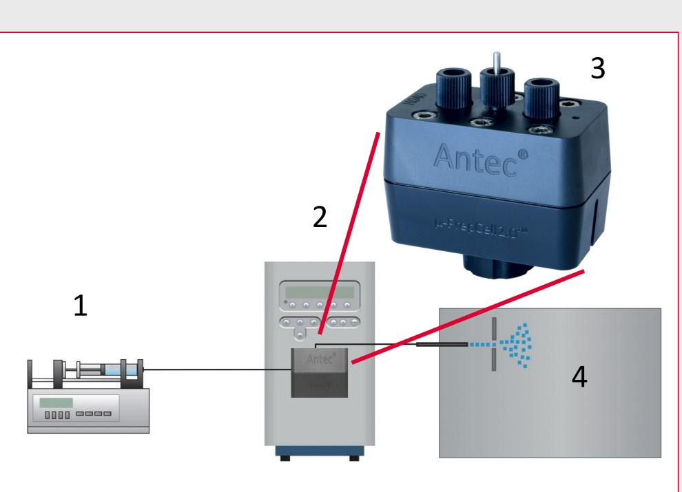
Figure 1: Schematics infusion Electrochemistry/MS system: 1) Infusion pump, 2) ROXY Potentiostat equipped
