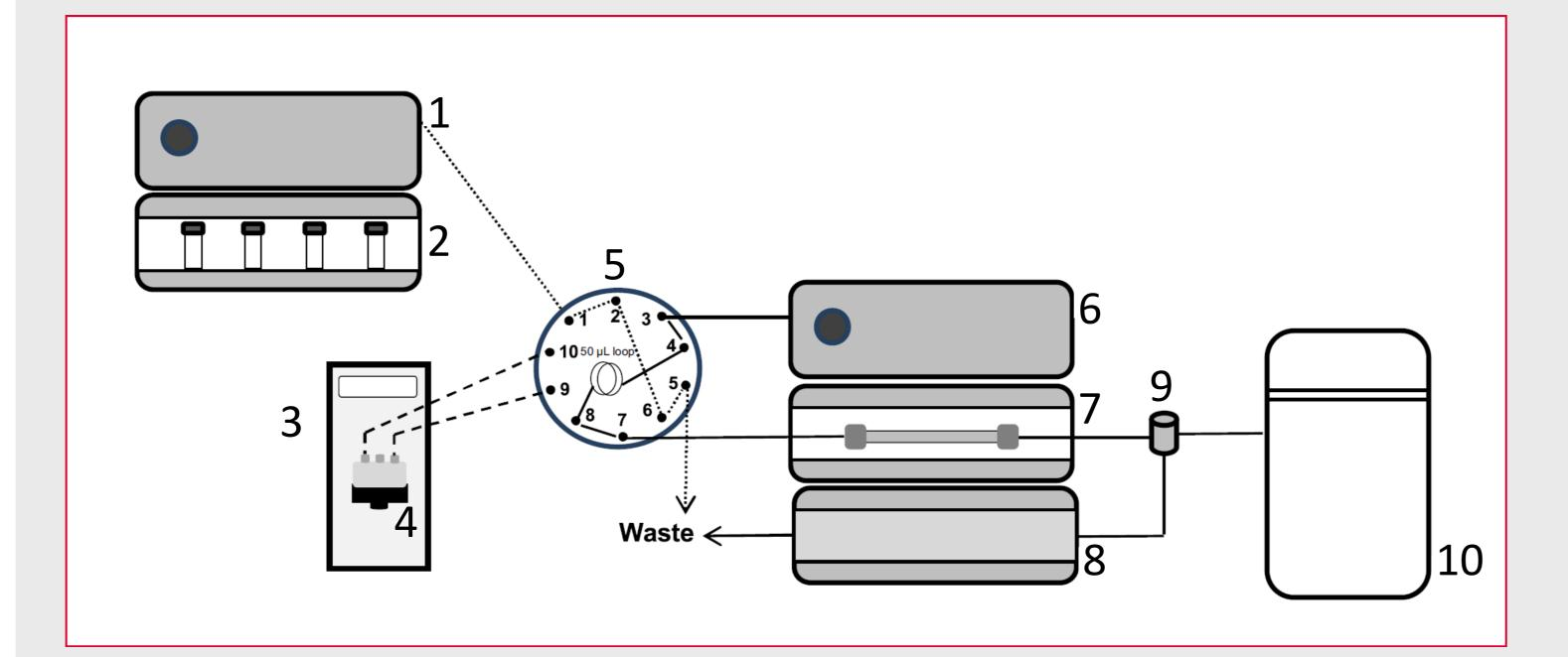
Figure 2: Schematics of automated on-line EC-LC-UV-MS system used to study the oxidative behavior of **drug compound**. 1) loading/washing pump, 2) autosampler, 3) Roxy potentiostat, 4) electrochemical cell (μ-PrepCell), 5) 10-port switching valve, 6) gradient pump, 7) column compartment, 8) UV detector, 9) flow splitter, 10) MS
