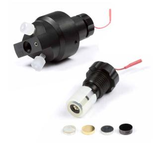
(MD), which can be quickly and easily exchanged. Magic Diamond (MD) also known as Boron Doped Diamond (BDD) is the workhorse and electrode of choice for oxidation reactions up to a maximum applicable voltage of 4.0 V. Pt and Au are typically employed for specific reactions such as hydroxylation or N-oxidation.
