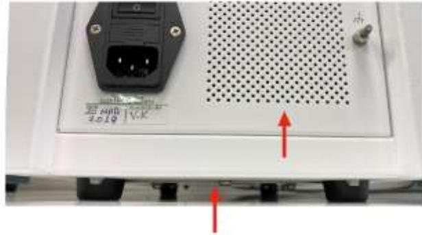
Fig. 2. Location of ventilation holes in the DECADE Elite (bottom & rear).
