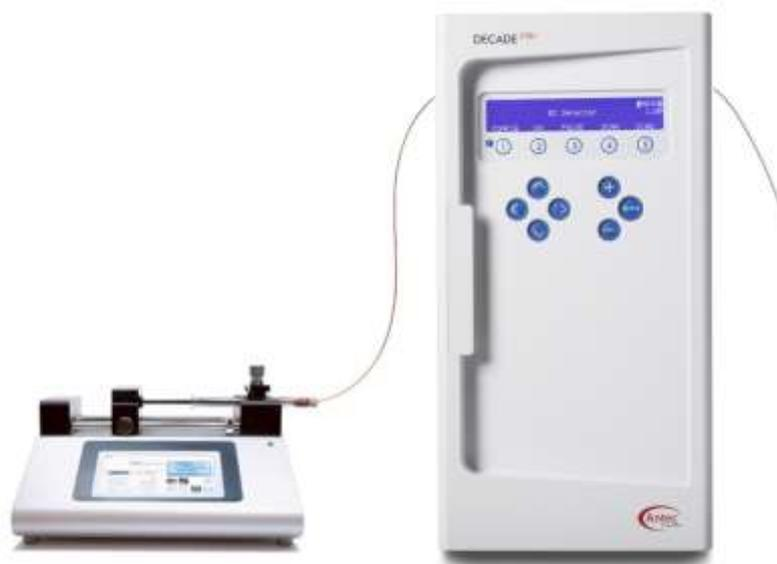
Fig. 53. DECADE Elite scanning voltammetry set-up with a syringe pump.
