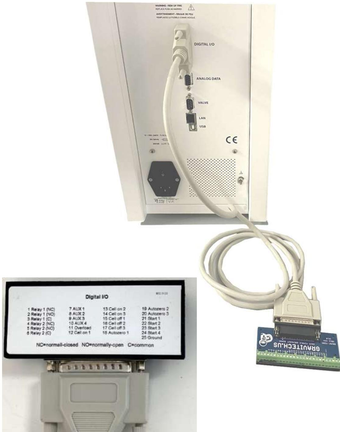
Fig. 70. Top: DECADE Elite with I/O screw terminal board installed. Bottom-left: back side of screw terminal board.
