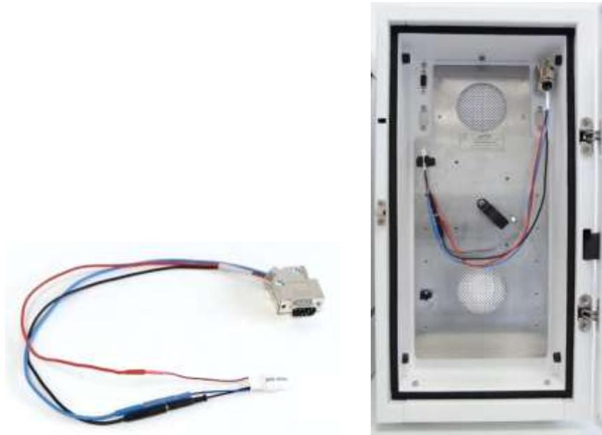
*Fig. 73. Left: cell cable with external dummy flow cell (pn 250.0040). Right: detector with external dummy flow cell.*
